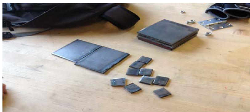
Figure 4: square sections for leveling pads
