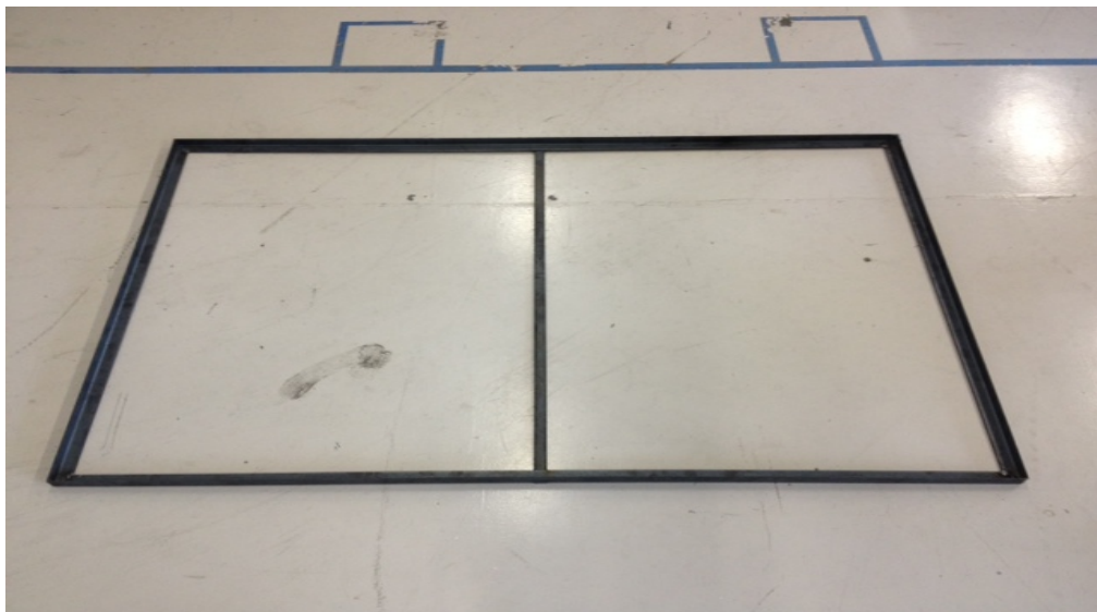
Figure 1: Solar Panel Frame.
