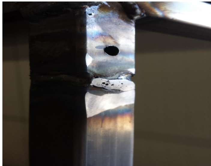
Figure 2: Fixed welded joint for square tubing
